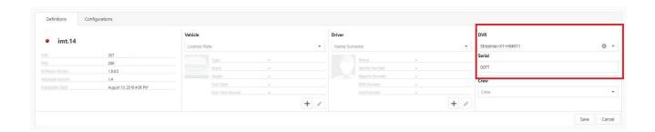
Click on arrow to the left of the Device ID to match. Select the DVR model on the right of next screen, fill in Serial No. and Save.
